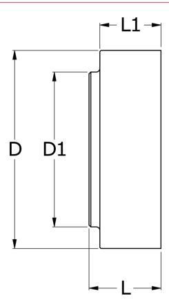
$\begin{array}{lll} D & = 520 \\ D1 & = 315 \\ L & = 210 \\ L1 & = 102 \\ Max bore & = 190 \\ Torque (N m) = 21200 \end{array}$
